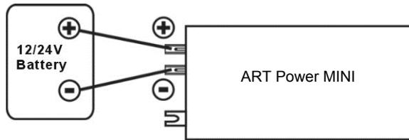
In addition, the batteries can be wired to provide additional run time. The various wiring configurations are as follows:
